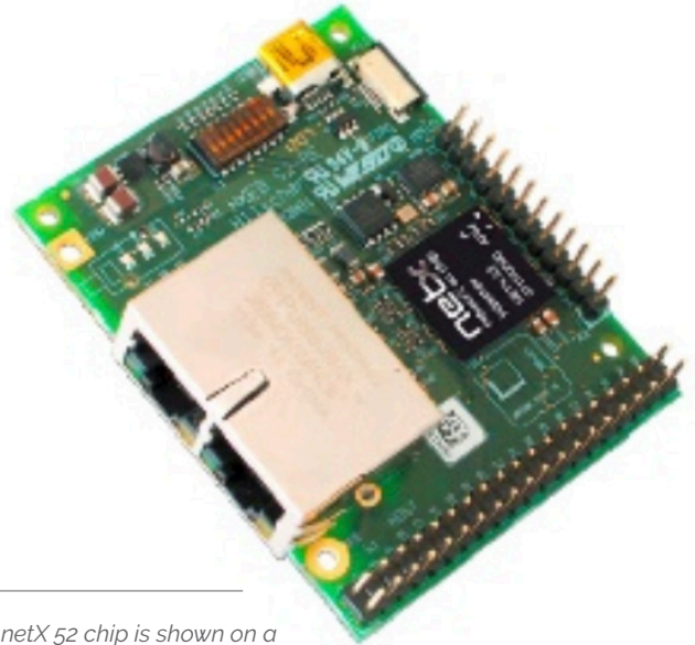
The netX 52 chip is shown on a typical network adaptor board.
