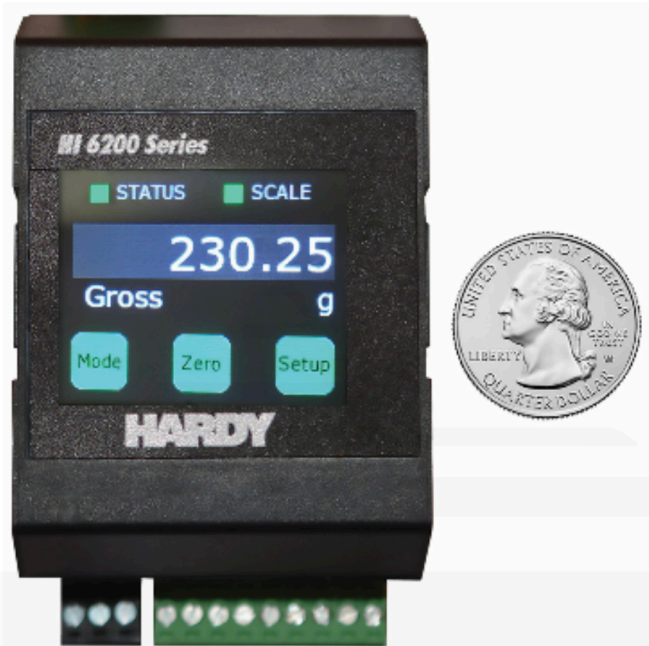
Figure 1: The HI 6200 single channel weight controller/indicator has been upgraded to support PROFINET using Hilscher's netX 52 networking chip.
